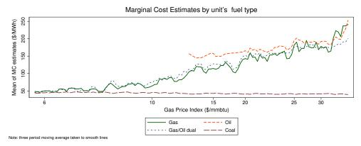
*Notes*: Unit-specific marginal cost estimates of days in Sample 1 are averaged within each fuel type categories: gas, oil, dual, and coal. The set of units included in the calculation of the average value changes over time. Averaged estimates are plotted against the gas price index values of the days in the sample.
