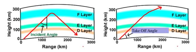
Figure T.4: Maximum usable frequency (MUF)
