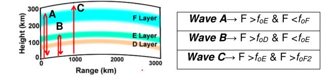
surface. On the basis of this phenomenon it is possible to define the *critical frequency*,  $f_o$ , of an ionospheric layer such as the threshold frequency above which an EM wave (incident at 90 degrees), passes through the object in the layer without being refracted towards the ground. Each ionospheric layer has its own critical frequency, defined as follows:
