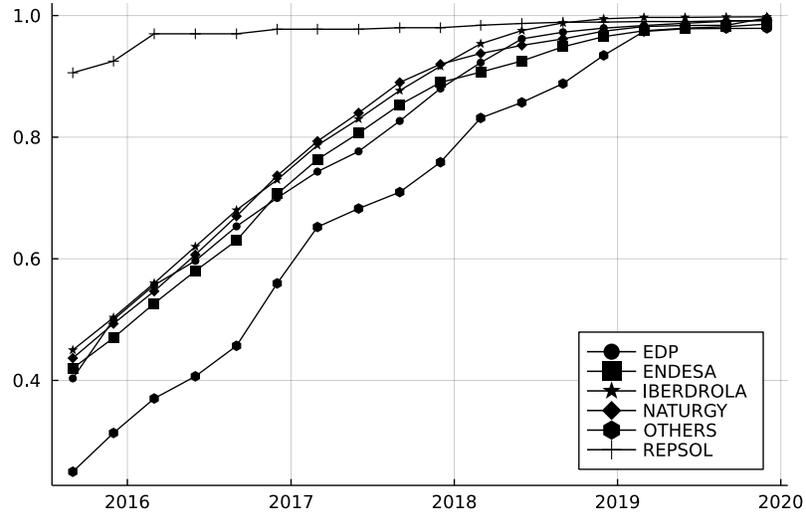
Figure C.1 shows the smart meter deployment in each distribution area. In mid-2015, all 5 traditional distributors had a coverage of around 40%, except for Repsol (before Viesgo) which had a coverage as high as 90%. By 2019, universal coverage was reached in all distribution areas.
