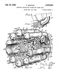
Whittle's 1940 Engine: 950 pounds, 2187 horsepower, about 50 labeled parts
