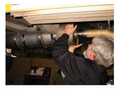
Figure 3: Installation of diesel particulate filter on DeKalb bus prior to testing.
