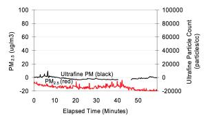
Figure 2: The DPF-ULSD-Spiracle combination eliminated PM<sub>2.5</sub>, ultrafine particles, black carbon, and PAH self pollution from the bus cabin. Ambient concentrations have been subtracted resulting in slightly negative apparent net concentrations. Concentrations below zero should be taken as zero net PM<sub>2.5</sub> contribution to the bus.
