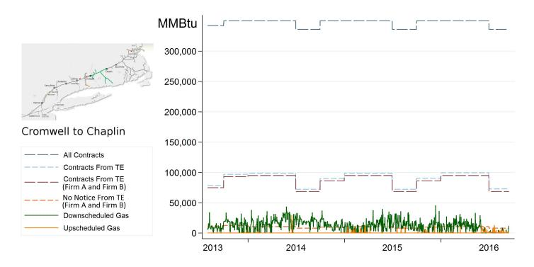
Figure 8: Aggregate downscheduling behavior compared to the contract positions of Firms A and B over time within pipeline's "J System," which serves many large electricity generators as well as a substantial heating market. Two regularly withholding nodes are located here. There is no clear correlation here between aggregate downscheduling and contracts held by Firms A and B.
