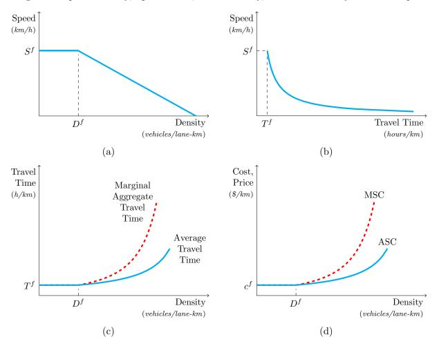
Figure 1: Speed-Density, Speed-Time, Time-Density, and Cost-Density Relationships
