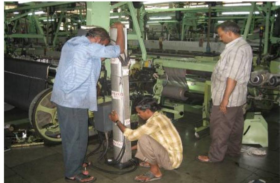
Loom parts being disassembled for diagnosis
