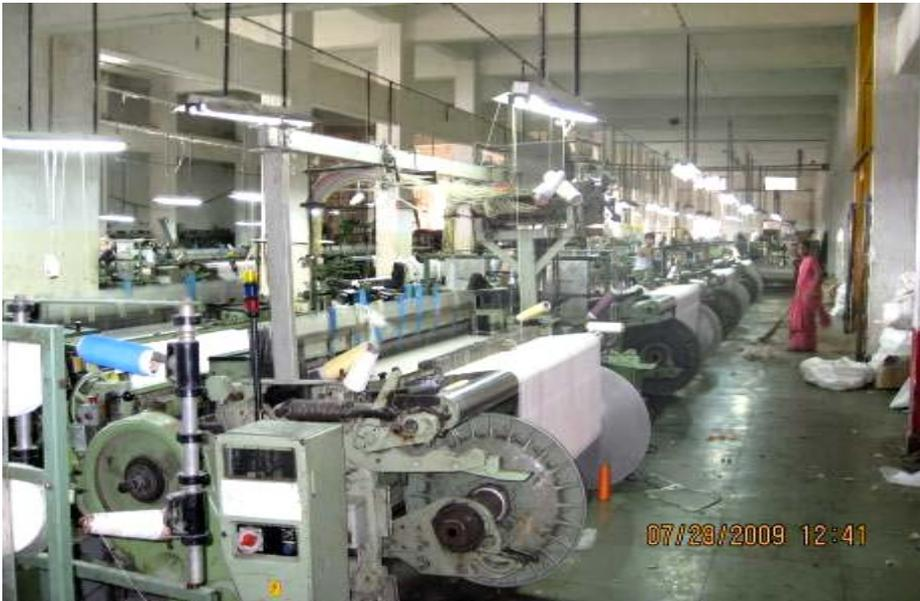
(3) Weaving the fabric on the weaving loom
