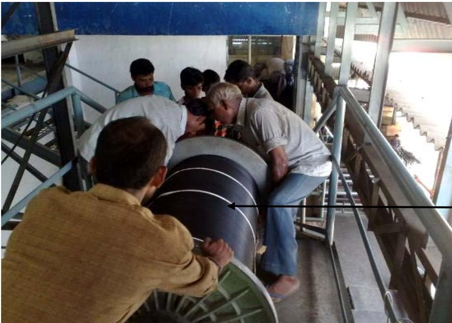
At another factory both warp beam elevators had broken down due to poor maintenance. As a result teams of 7 men carried several warps beams down the stairs every day. This was slow and dangerous, with two serious accidents in our time at the factory.
